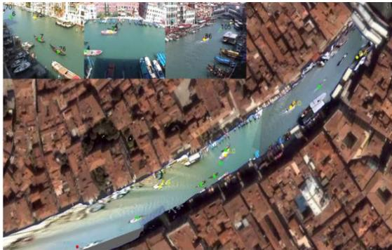
Figure 11: Multi-camera data fusion example: three camera frames are rectified and stitched into a composite image [37].
