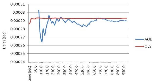
Fig. 3 Host-to-Host delays 16 nodes AODV vs. OLSR attacks
