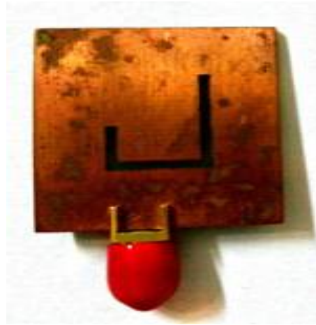
Figure 7: Prototype of Reconfigurable Antenna (Back View)
