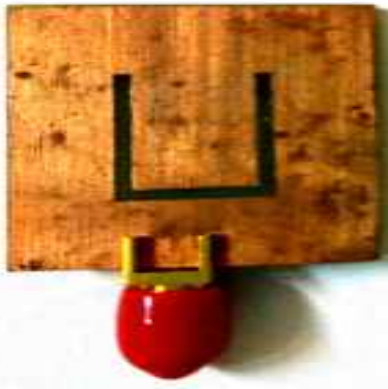
Figure 5: Prototype of Triple Notch Band Antenna (Front View)
