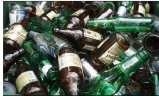
**Figure 1:** Waste glass bottles as collected before crushing and sieving
