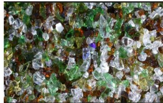
**Figure 2:** Crushing of glass bottles to coarse sizes
