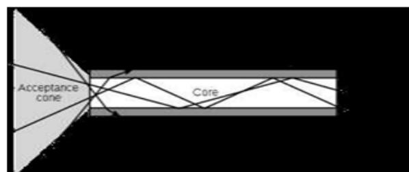
**Figure 9** Total internal reflection
