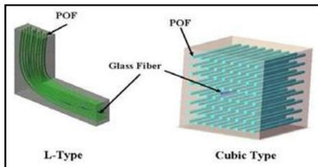
**Figure 1** Integrated model of translucent concrete cube
