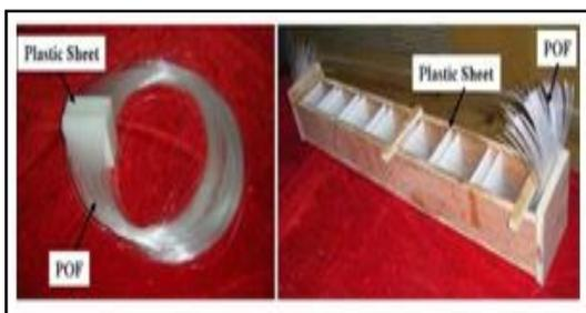
**Figure 2** Form-work of wood and thermocol
