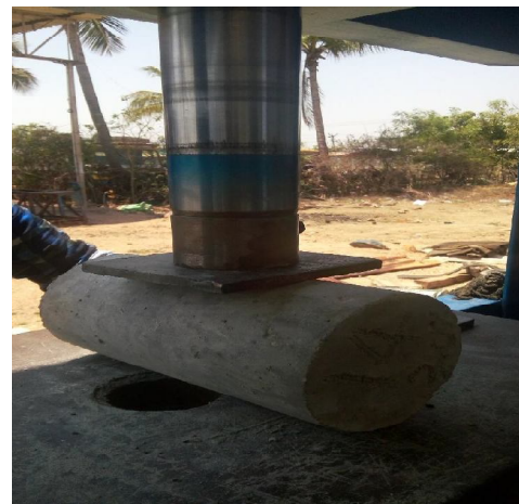
Figure 5 Split tensile test setup
