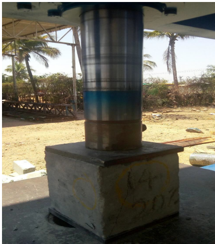
Figure 4 Compressive strength test setup
