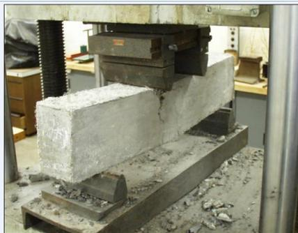
**Figure 3** Flexural strength test
