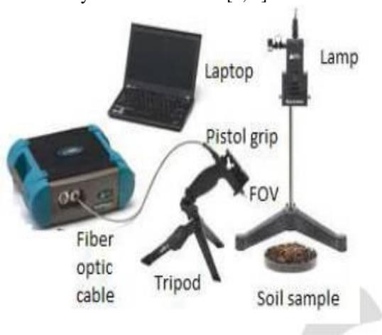
**Figure 2.2** working of ASD FieldSpec 4 Standard-Res Spectroradiometer.
