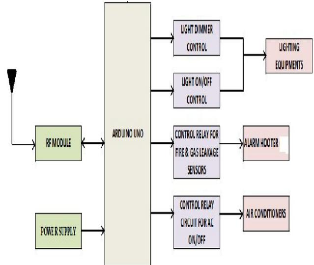
Figure 3 Block Diagram for Receiving Unit
