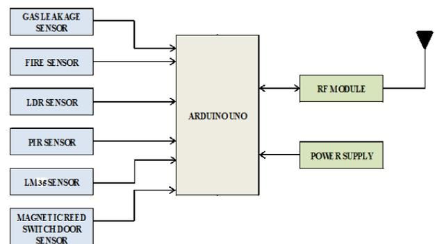
Figure 1 Block Diagram for Sensing Unit
