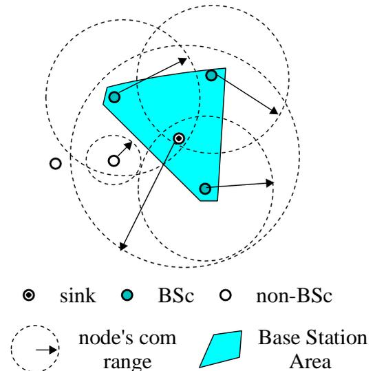
Fig. 1: The base station area.
