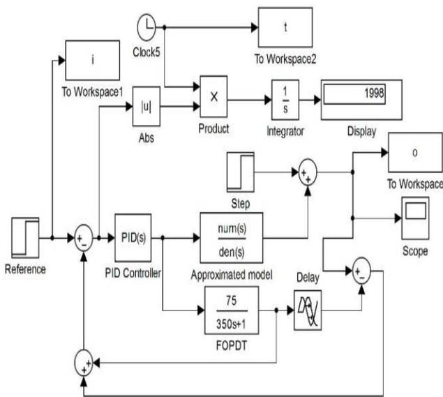
Figure 12 Simulink model of S-P PID controller
