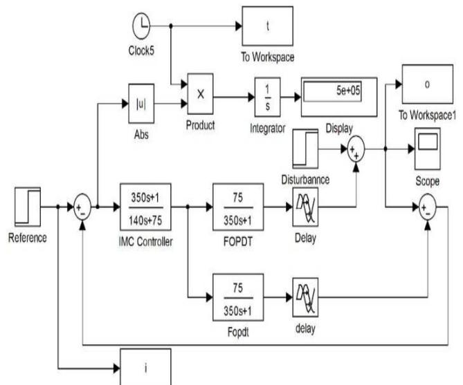
Figure 14 Simulink model of IMC controller
