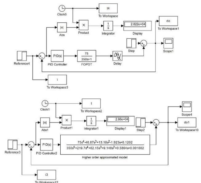
Figure 11 Simulink model of Z-N PID controller
