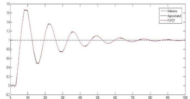
Figure 10 Closed loop response of FOPDT & pade model
