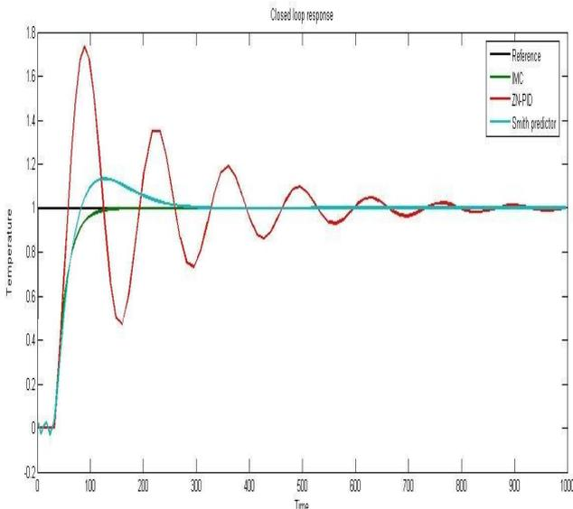
Figure 15 Closed loop response
