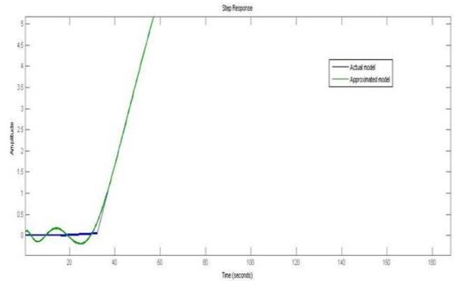
Figure 9 Step response of FOPDT and approximate model
