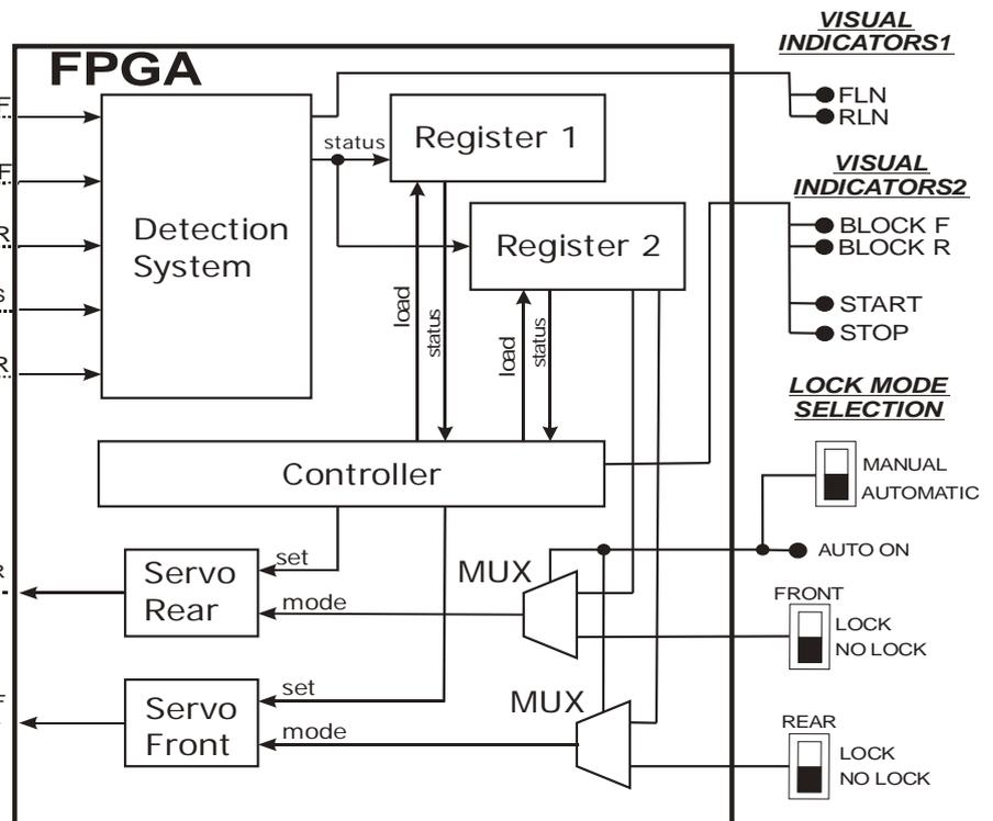
**Figure 3** Block diagram of the Locker control system
