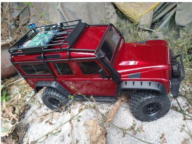
**Figure 9** Traxxas TRX-4 with differential control system
