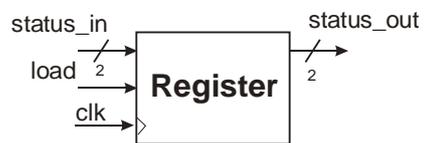
Figure 5 Input and output signals of the register block
