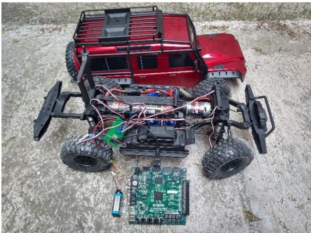
**Figure 8** Traxxas TRX-4 and FPGA Board
