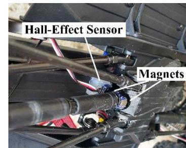
**Figure 2** Bottom-view of vehicle showing driveshaft sensor and magnets
