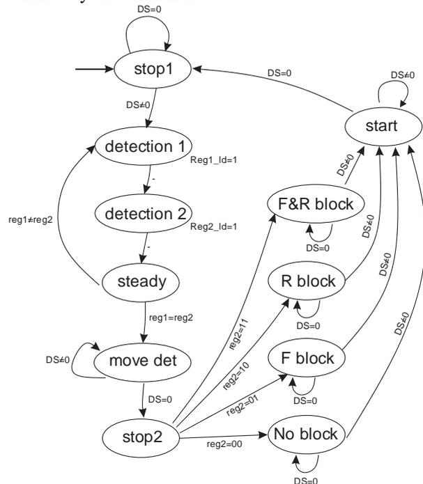
Figure 6Finite-State Machine of the controller
