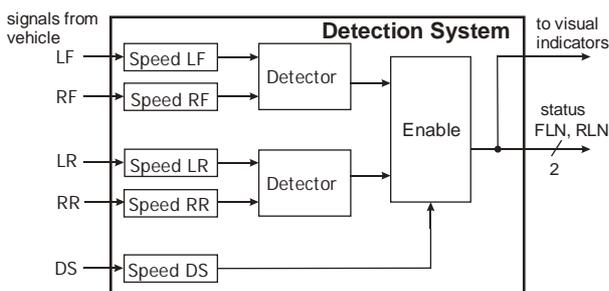
Figure 4 General block diagram of the detection system
