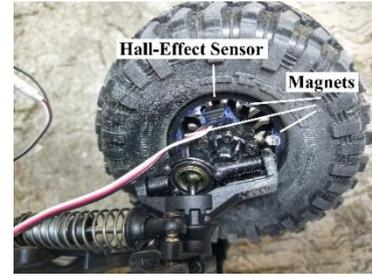
**Figure 1** Right front wheel and suspension with Hall-Effect Sensor and Magnets
