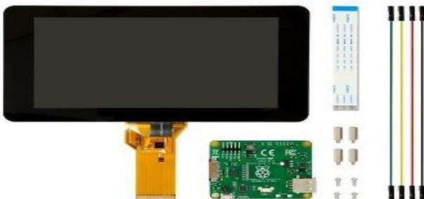
Fig.4 7"Official Raspberry Pi Display with Capacitive Touch screen [13]
