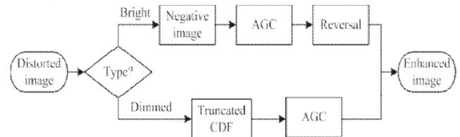
Fig.1 Flowchart of the gamma correction based method[1]
