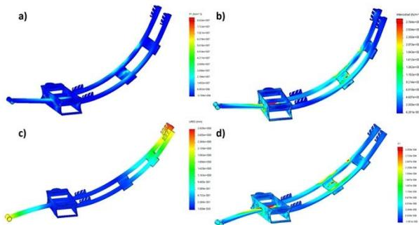
Figure 8 Finite element model outputs: (a) Principal normal stress distribution. (b) Principal shear stresses. (c) Maximum deformations. (d) Principal normal strain distribution
