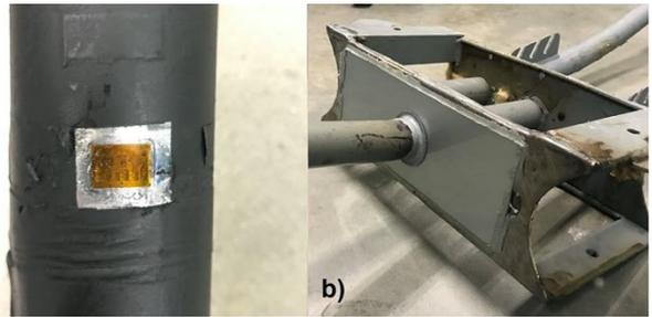
**Figure 6** Installation process of (a) rosette and (b) photo-elastic plate used in the validation of the HPV structure
