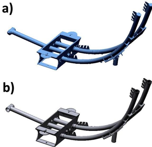
**Figure 3** (a) 3D-scanned model in Geomagic Design X software. (b) 3D-solid geometry imported into Solidworks software, ready for simulation using finite element analysis
