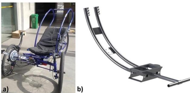
**Figure 1**(a) Human-powered vehicle (HPV) and (b) Mainframe of the chassis used for the HPV
