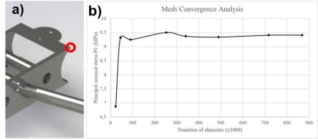
Figure 9 (a) Node of analysis for the verification process and (b) mesh convergence test results
