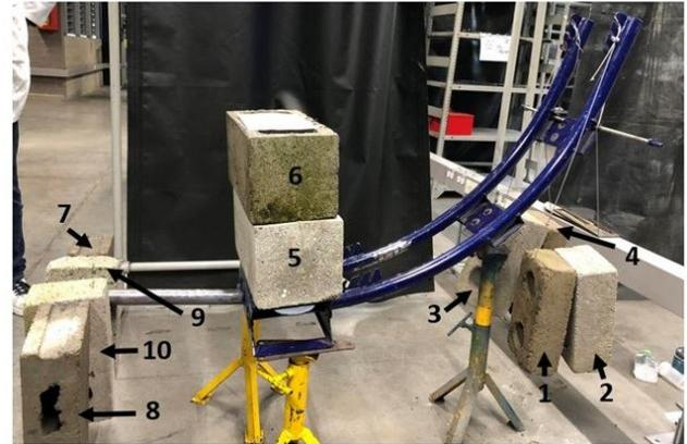
**Figure 2** HPV physical model loaded with bricks simulating the operational critical load condition
