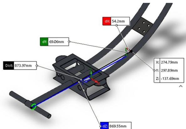
**Figure 5** Position of the point of analysis with respect to the frontal tube end; relative coordinates are with respect to the global coordinate system. Overall distance is in black, while the component distances parallel to the X-, Y-, and Z-axes are respectively labeled in red, green, and blue
