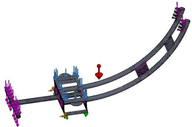
**Figure 4** 3D model within the FEA software with the material applied, initial meshing, boundary conditions defined, and loads applied. The color convention in the graph is as follows: magenta for anterior and posterior loads, pink and green for displacement restrictions, blue for central load, and red for gravity load exerted on the model
