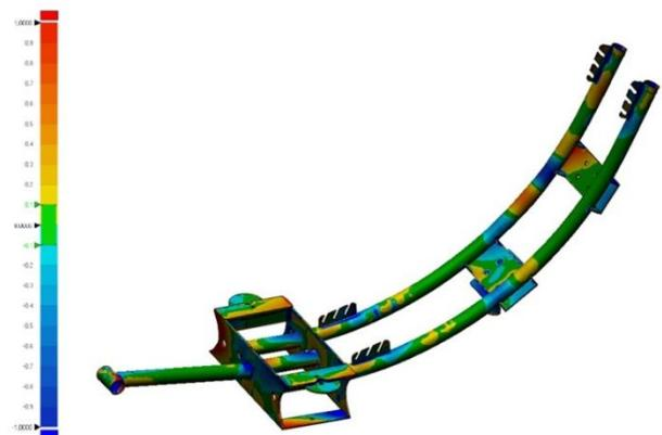
**Figure 7** Deviation analysis of the reconstructed mesh with scale in mm. Regions extending beyond the original scanned geometry are marked in red while regions lying below the original geometry are marked in blue. In both
