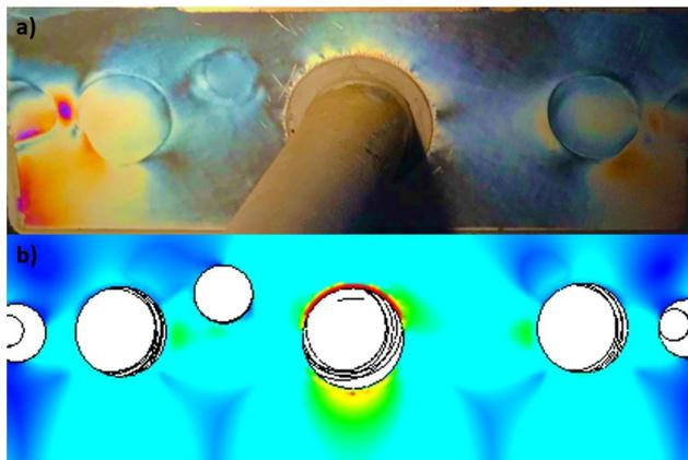
**Figure 11** Similarity between (a) the numerical model results for strain distribution and (b) the photo-elastic physical stress patterns
